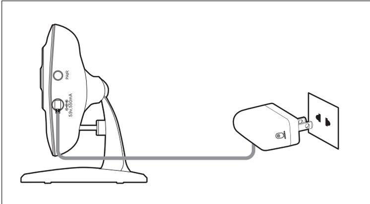
1. Connect the Camera Power Adapter to the Camera Unit.
