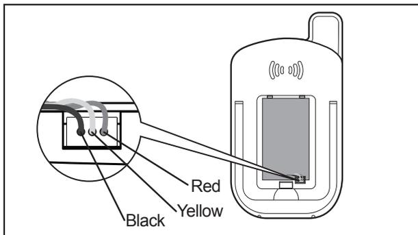
1. Insert the Rechargeable Li-ion Battery into the Battery Compartment as shown above.
